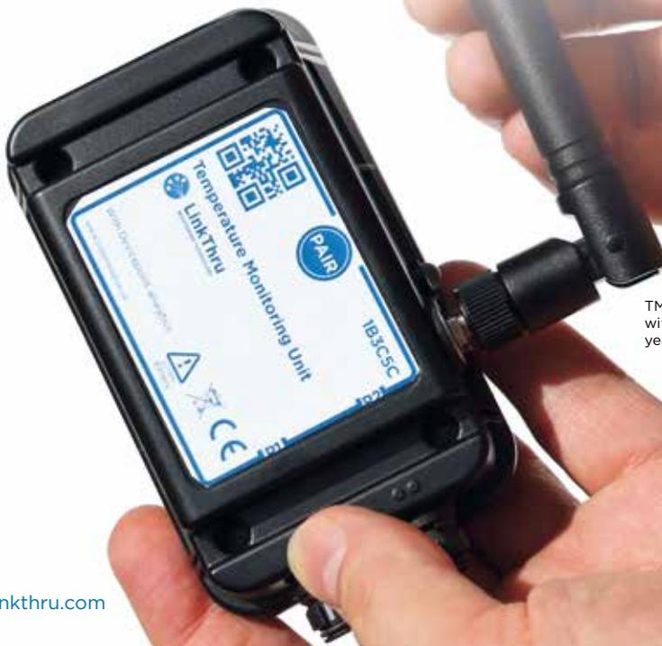
TMU devices are battery-powered with a long life of between 3 and 5 years, depending on the data mode.
