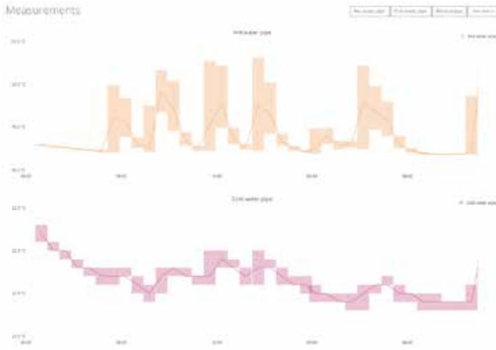
This example dashboard screen shows monitoring of hot and cold temperatures over a two-day period.
